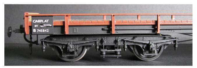
11. Fit vacuum cylinder and associated castings, using the short 1.2mm rod for shafts and with the 13 hole adjusters (pointing towards the bogie!) above the shaft when the wagon is the correct way up. The 13 hole adjusters should be drilled 0.9mm and a length of wire added after the bogies have been fitted. One end has a full width shaft for the handbrake
