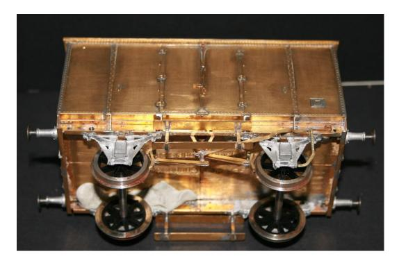
12. Fit V hangar (17) to the inside of the solebar with the rivets – using the etched centreline to position correctly. Add inner stirrup (18) with pivot casting (tumbler) loosely located in the holes.
