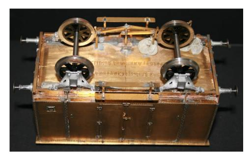
14. Form brake lever (31) as shown below and fit with ratchet to solebar. The distance of the ratchet from the axle centreline = 6mm (to the right). Note, the two half etch dots are the centres of the reverse bends NOT fold lines. Part 32 fits over the protruding spindle of the tumbler casting.
