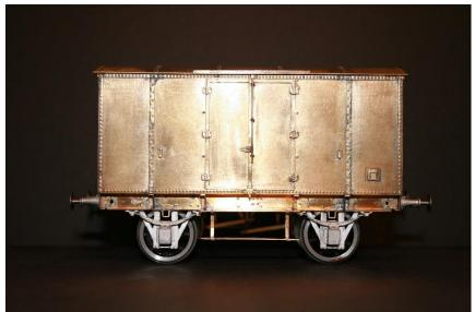
7. The roof (23) should be curved to match the ends and the rivet detail strips (25) added. The gutters fold so that they are horizontal and at 90 degrees to the body side when the roof is in place. Rainstips (24) fit in the half etch line. See photos below. The roof can be fitted now or left until after painting
